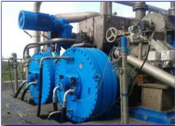
Twin Roll Wash Press Drive for Pulp & Paper Industry
