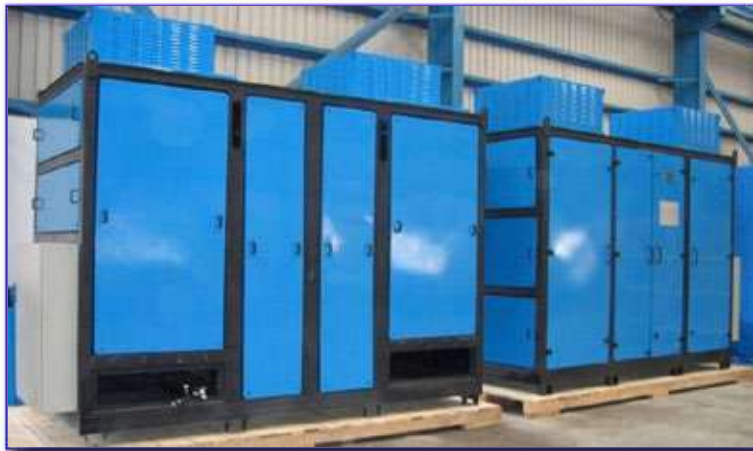
Tandem Drive – Vertically Mounted Pump-Motors Front & Rear Views of Sound-Proof Cabinets
